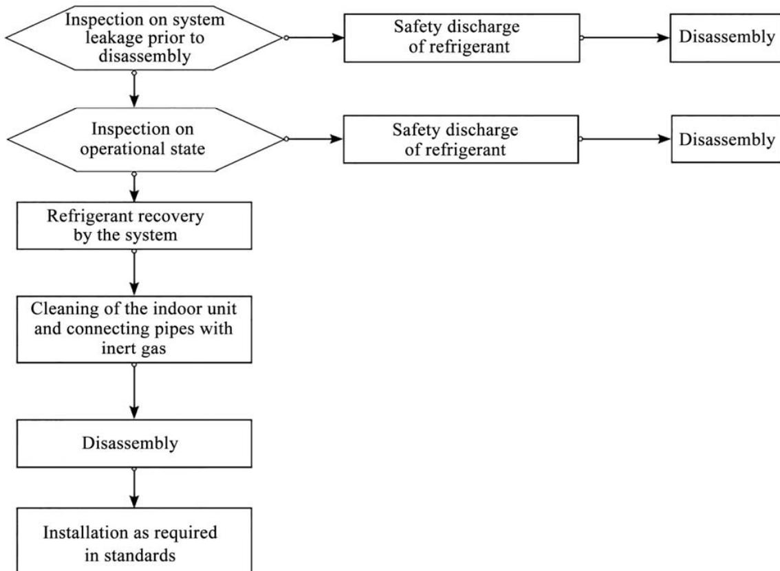
Note: In case relocation is required, the joint of evaporator gas/liquid pipes of the indoor unit shall be cut off with a cutting knife. Connection is only allowed after re-flaring (the same to the outdoor unit).
