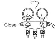
4. Open the valve for the 2-way valve to an angle of anticlockwise 90 degree. After 6 seconds, close the 2-way valve and make the inspection of gas leakage.
