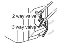
7. To prevent the gas leakage, turn the service ports cap, the valve rod's cap for 2-way valve and 3-way's a little more than the point where the torque increases suddenly.
