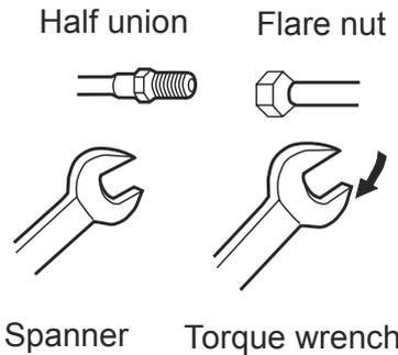
Forced fastening without careful centering may damage the threads and cause a leakage of gas.
