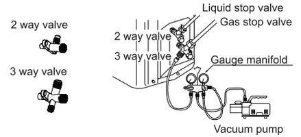
2. Open the handle at low in gaugemanifold, and operate vacuum pump. If the scale-moves of gause (low) reach vacuum condition in a moment, check the step 1 again.
