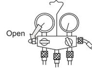
3. Vacuumize for over 15min. check the level gauge which should read - 0.1MPa (-76 cm Hg) at low pressure side. After the completion of evacuation , close the handle 'Lo' in the vacuum pump. Check the condition of the scale and hold it for 1-2min. If the scale-moves back in spite of tightening, make flaring work again, then return to the beginning of the step 3.
