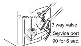
5. No gas leakage? In case of gas leakage, tighten parts of pipe connection. If leakage stops, then proceed the step 6. If it does not stop gas leakage, discharge whole refrigerants from the service port. After flaring work again, fill up prescribed refrigerant from the gas cylinder.
