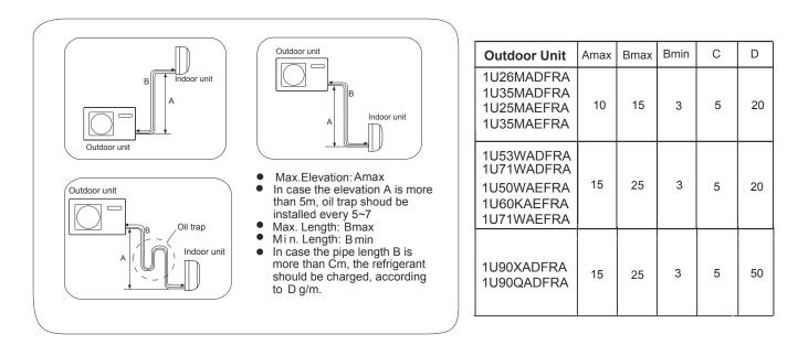
After finishing connection of refrigerant pipe, it shall perform air tightness test.
