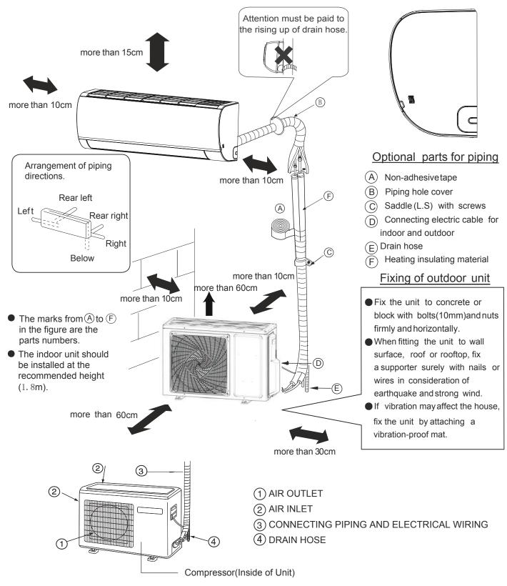
1. When installing the unit to wall, roof or rooftop, fix a supporter surely with nails or wires in preparation of earthquake and strong wind.
